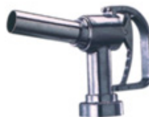
JY1295 (Manual Nozzle) Inlet:PF1 1 / 2 "2"-11gear, PF2 1 / 2 "-8gear, Outlet: 1 1 / 2 " Flow rate: 0-290L/M Pressure: 0.18Mpa
